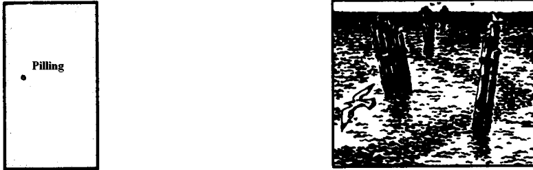
Figure 99. Dolphin, Piling, Stump, Snag. Appropriate labeling indicates the type of obstruction.
