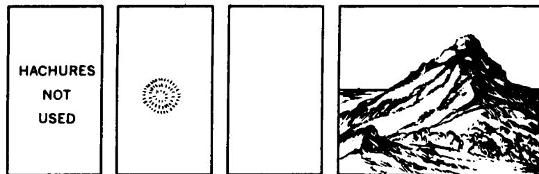
Figure 43. Hachures. This symbol is used to indicate significant formations not revealed by contours.
